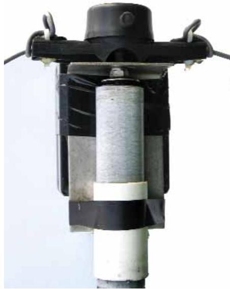
PHOTO 3: Close-up of the rotating dipole centre (balun box to the rear).
